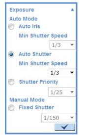
The exposure is the amount of light received by the image sensor and is determined by the width of lens diaphragm opening, the amount of exposure by the sensor (shutter speed) and other exposure parameters. With this item, users can define how the Auto Exposure function works.
