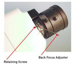
Step 2: Make sure the iris is wide open. Therefore, it is advised to keep the environment in low light condition. To open the automatic lens completely, please use a neutral density filter. With this filter it is possible to simulate a low light condition so that the lens can open up completely.
